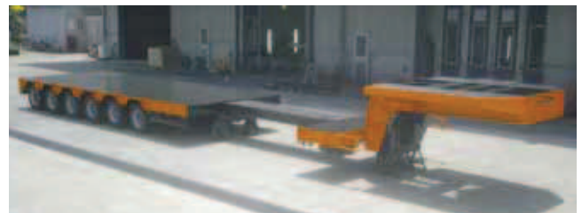
6-axle self-steering extendible semi-trailer Semi-trailer with allowable gross weight of 60 tons. The pallet is stretchable (3,5 meters) to carry large and heavy cargo up to 55 tons. The steering mechanism enhances ability to turn and operate.
